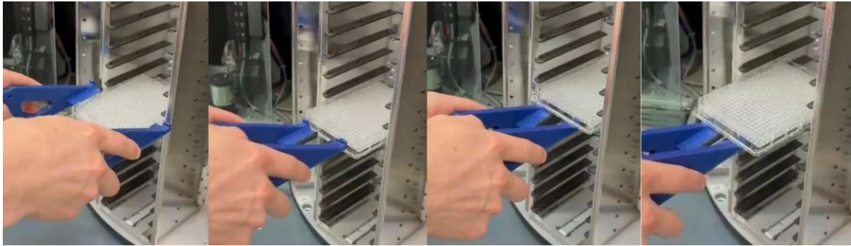
Figure 22: Motion for placing and taking plates from plate hotels with gripper 3.1 iteration
